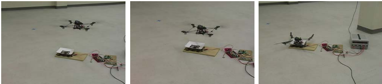
Figure 7: Fully Autonomous Landing and Recharge Demonstration
