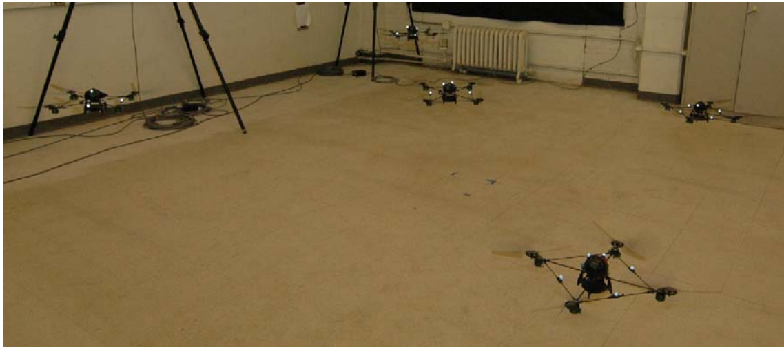
Figure 1: Five Autonomous Vehicle Flight Test using RAVEN's Autonomous Mission Manager
